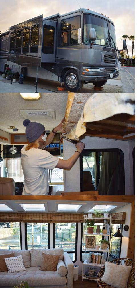
hadn't disclosed and even covered up a lot of water damage. They ended up having to replace the entire subfloor and ceiling in the back half of the RV.
